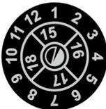
The inspection plate on the device shows confirmation of the last maintenance and the next scheduled maintenance.
