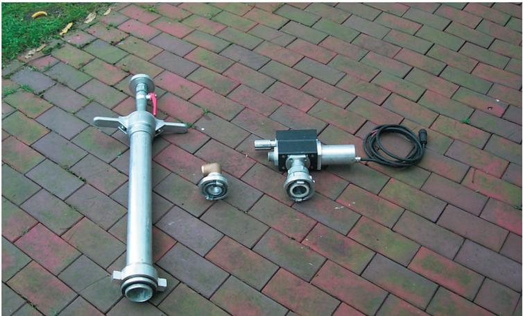
Picture 11: Stopper, stand pipe, flushing adapter
